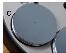
Collection substrates: a) multi-well plate; b) liquid vial; and c) silicon wafer on SEM stub.
