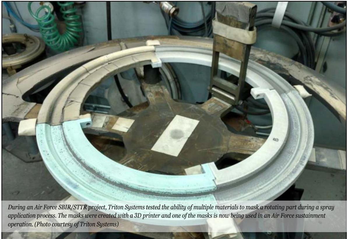
*During an Air Force SBIR/STTR project, Triton Systems tested the ability of multiple materials to mask a rotating part during a spray application process. The masks were created with a 3D printer and one of the masks is now being used in an Air Force sustainment operation. (Photo courtesy of Triton Systems)*
