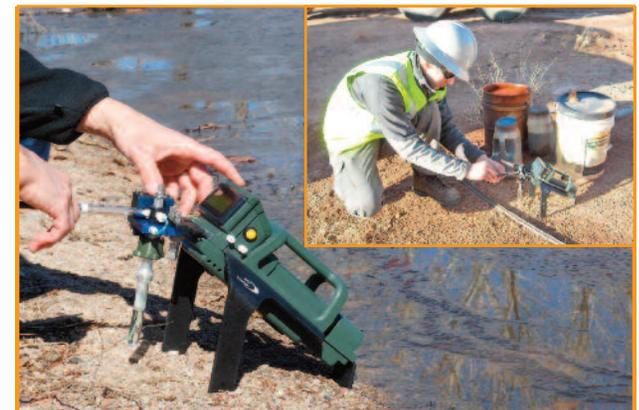
The portable FROG-4000™ expedites chemical detection and analyses of volatile organic compounds (VOCs) in air, water and soil in real time.
